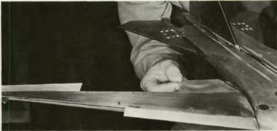
WING DAMAGE TEST. Tests to determine how long a damaged aircraft could remain in stable flight after the loss of wing-surface components help to determine combat survivability. Shown is a model of an F-111 wing with the leading- and trailing-edge flaps removed to simulate damage.
