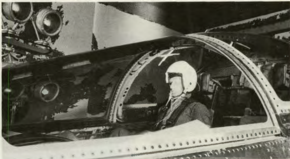
LAUNCH THE CHICKEN! In this special test an instrumented mannequin was used to study potential hazard to the aircrew of a high-performance aircraft subjected to a bird strike. The "X" above the mannequin's head marks the impact point in this pretest photograph. The test was sponsored by Air Force Flight Dynamics Laboratory.
